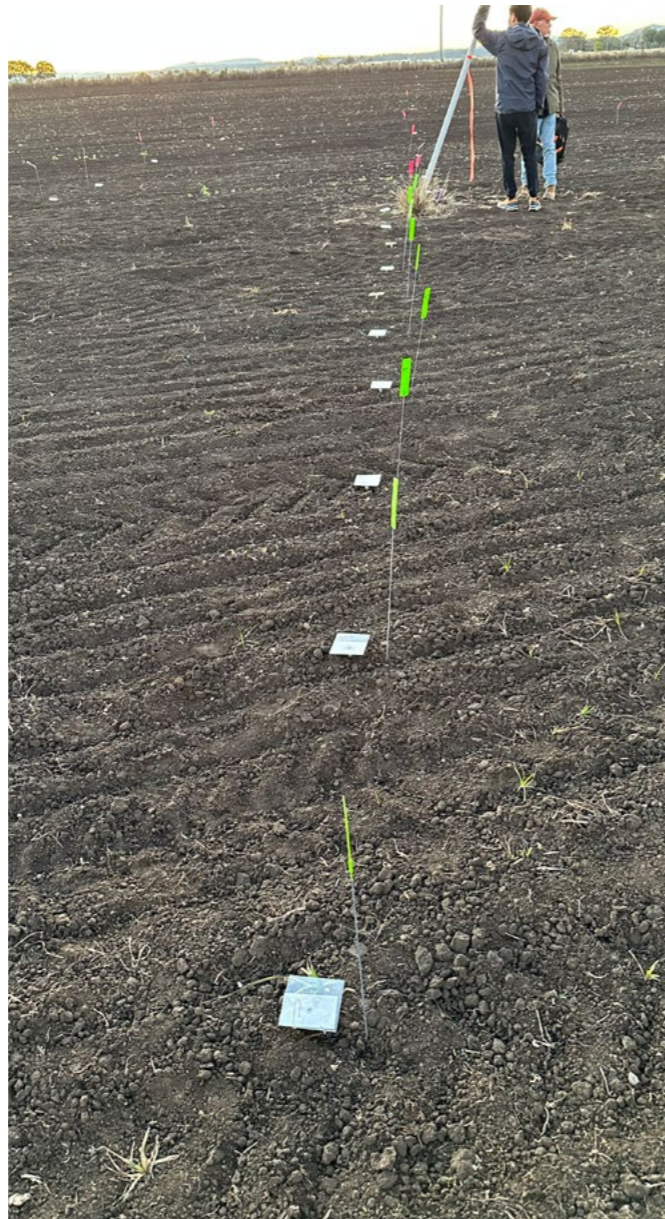
Ground droplet collection device
